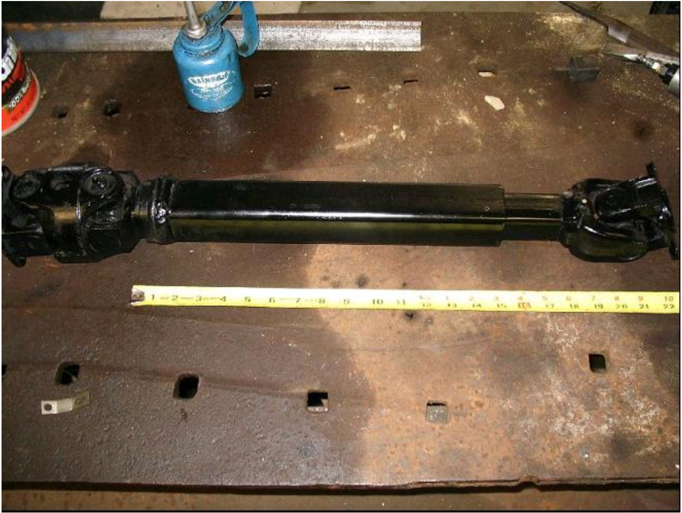
Figure 5. Driveshaft in normal driving configuration. Note the almost 3" of compression available.
