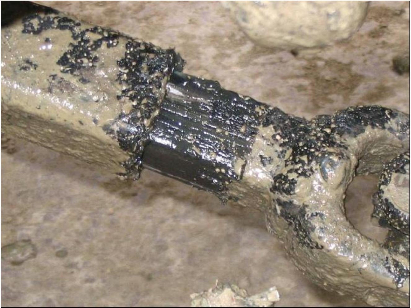
Figure 9. Driveshaft after extensive fourwheeling near Estill Fork, AL. Note that the grease path provides a good measure of the maximum compression of the driveshaft and that I still have \frac{1}{2} " – \frac{3}{4} " compression left although the front suspension was probably fully compressed at least once on this trip.
