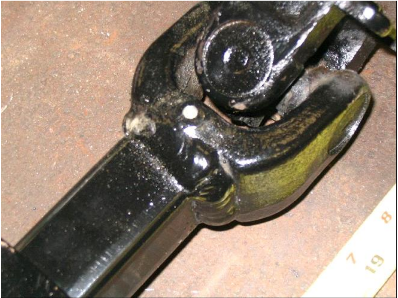
Figure 3. 1 ½" inner tubing welded to the yoke end. Note that the sides of the tubing are parallel with the yoke ears. The white hole in the center of the pic is the OEM grease fitting hole with some of the sand I added to the small tubing to help with balancing. After this pic was taken, I cleaned the hole up and welded it shut to prevent the sand from getting out.
