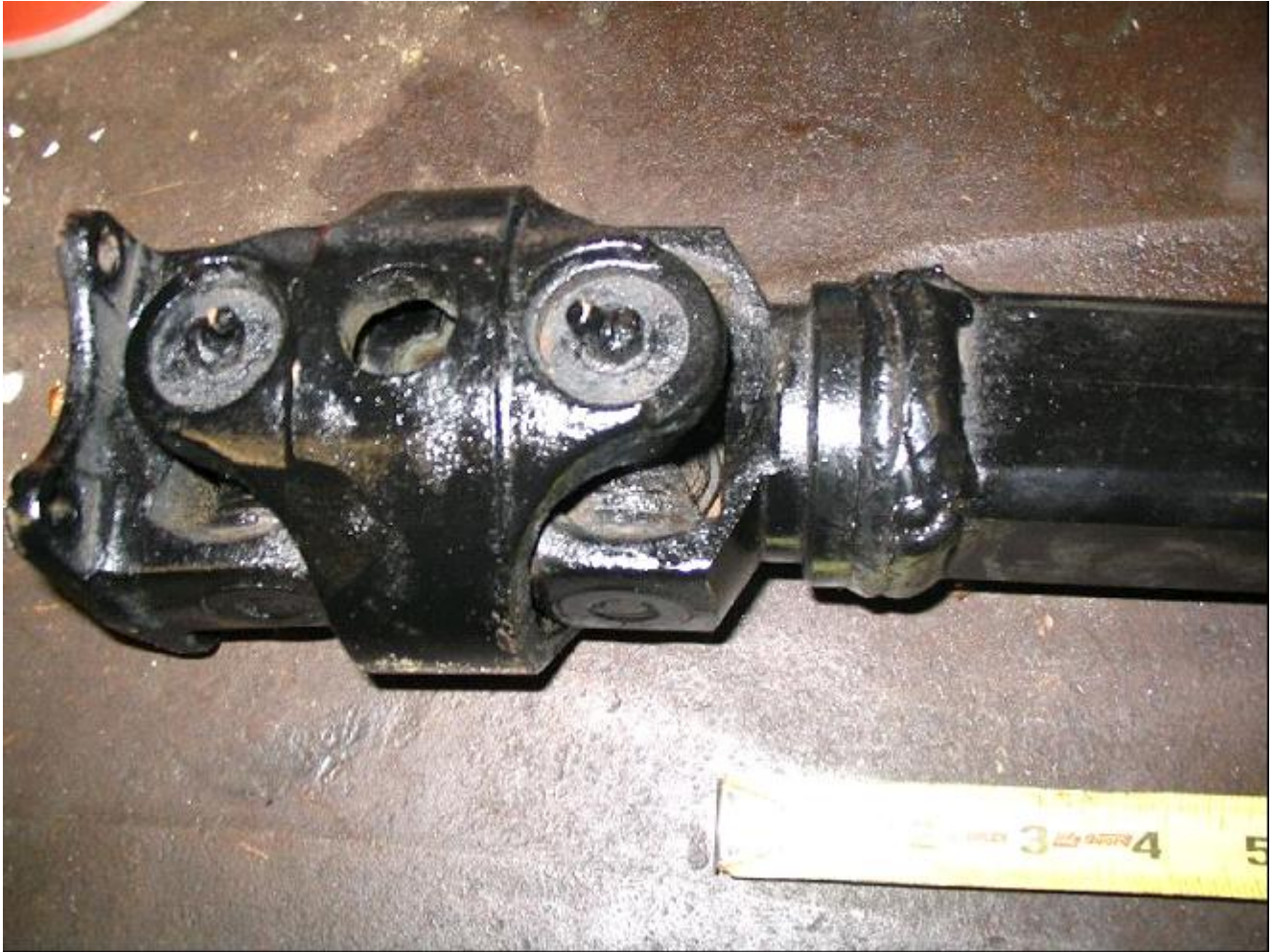
Figure 2. CV joint with 2" square outer tubing welded on the end. Note that the sides of the tube are parallel with the CV ears.
