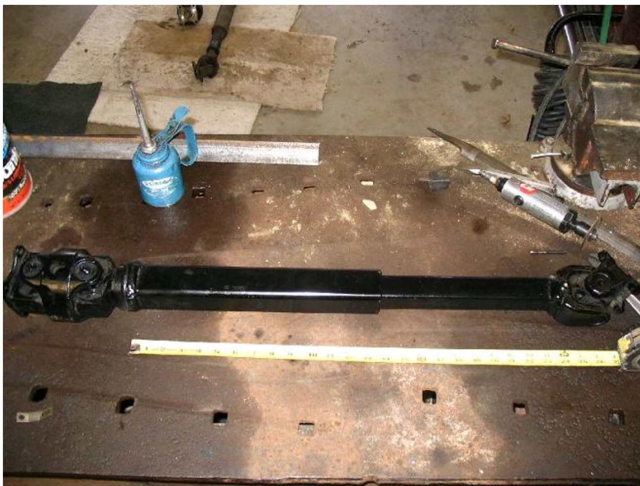
Figure 4. Final driveshaft in fully extended mode. Total extension distance is about 10"-11", compared to 2-3" (or less) for the OEM driveshaft. Note that the CV and yoke ears are in the same plane.
