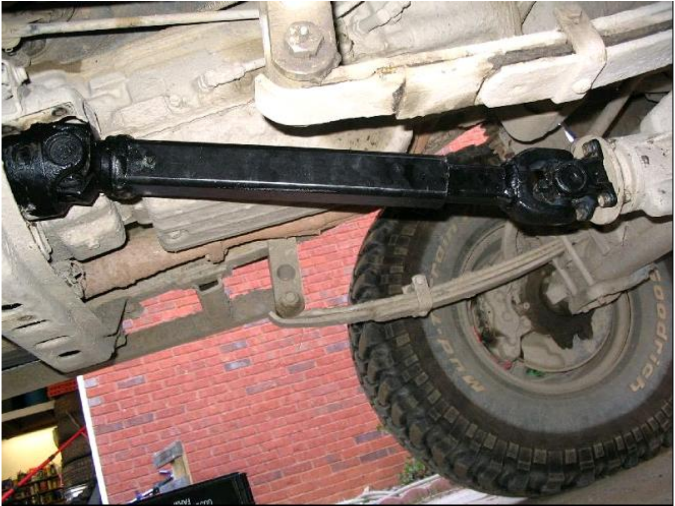
Figure 6. Driveshaft installed, vehicle sitting level in the driveway. Note the grease fitting near the CV end of the outer tube; this is to fill the outer tube with grease ensuring the two tubes can slide into one another without binding while on the trail.
