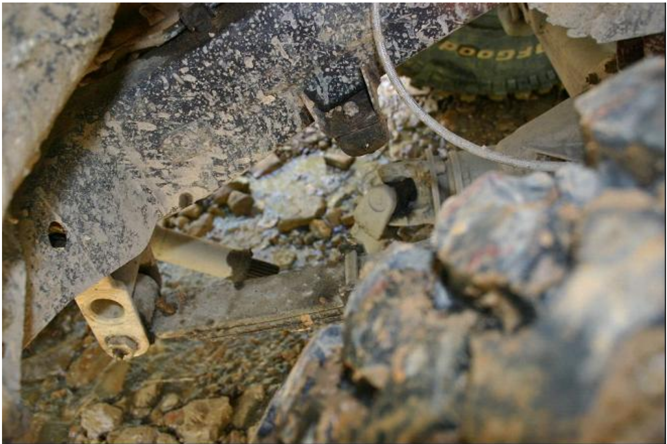
Figure 1. Front driveshaft separated but not damaged. Photo by Doc Elliott.
