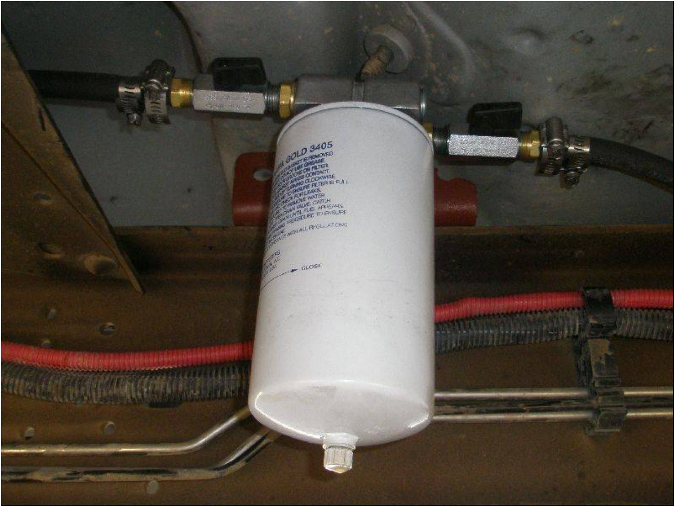
Figure 4. Wix 33405/Napa 3405 fuel water separator mounted under a 6.0l PSD; fuel flow is from left to right. Note the use of double hose clamps and 3/8" ball valves. The valves help prevent fuel leakage and loss while changing out the filter. You eyes aren't deceiving you: the filter head and filter are tilted slightly to the left. This was done to ensure the fuel line coming from the tank would clear the frame crossmember and keep the hose as straight as possible.
