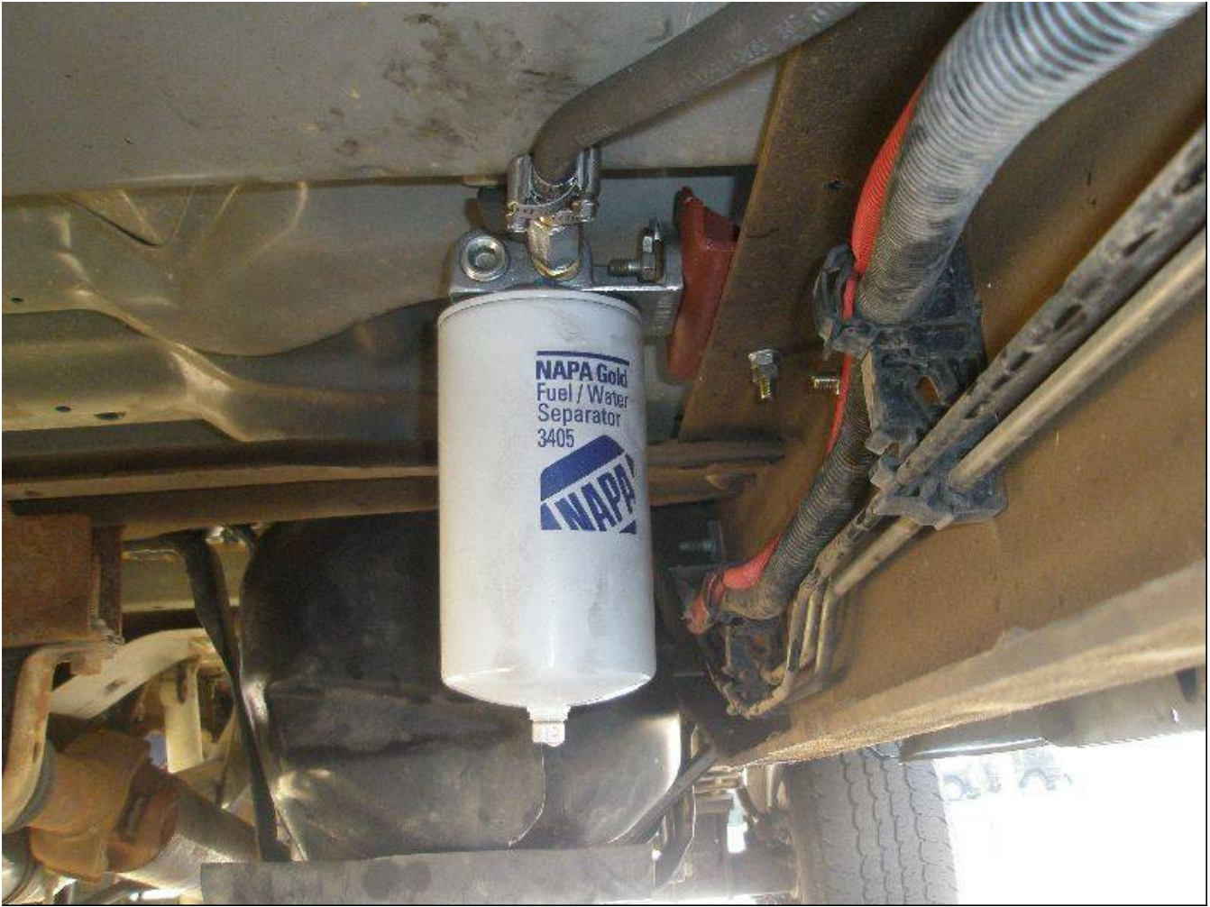
Figure 5. Wix 33405/Napa 3405 fuel water separator filter, Wix 24770/Napa 4770 filter head and mount. The bottom of the filter is just above the bottom of the frame, providing protection. The lower steel fuel line on the right center is the main OEM fuel supply line; note that it has been left stock.
