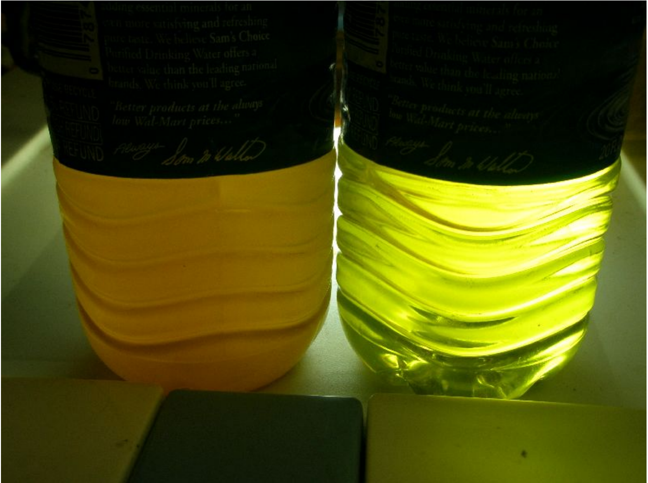
Figure 1. Two fuel samples recently drained from my 6.0l PSD. The sample on the left was drained from my aux fuel filter, the sample on the right, from the HFCM drain. Compare this pic with the FDDTS fuel samples in the article cited above. (Photo by author)
